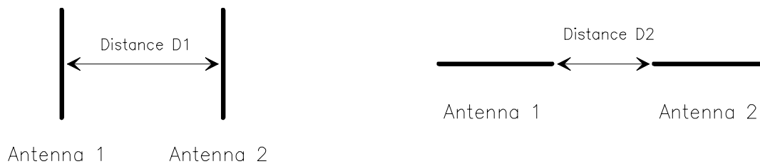
Figure 7: Distance between Antennas (top view)
